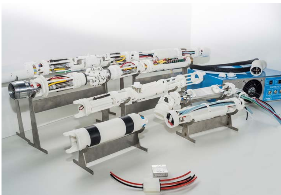
Fig.19 – The latest development of the 3D Prototype TORS system (75mm to 90mm)
