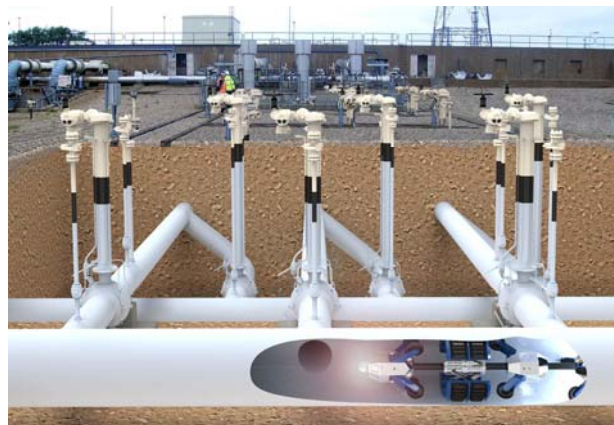
Fig.20 - Artists impression of Inspection Robot for unpiggable high pressure pipe lines
